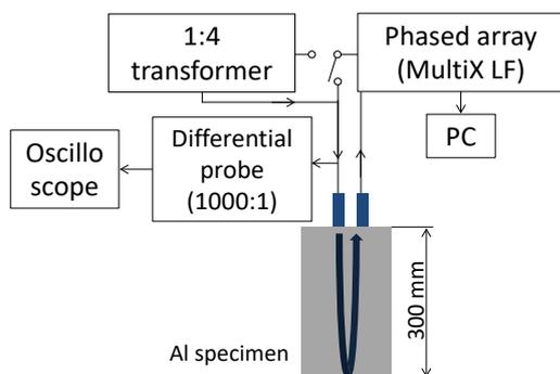
Fig. 3 Experimental configuration for measuring effective excitation voltage and bottom echoes.
