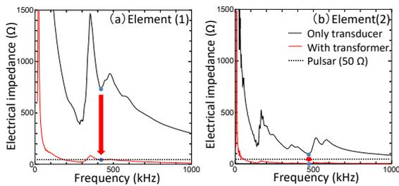
Fig. 2 Electrical impedance of elements (1) and (2).
