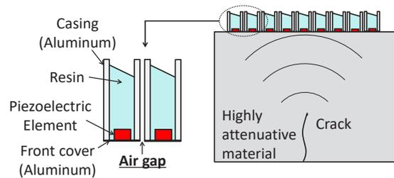
Fig. 1 LF phased array system with individual elements.
