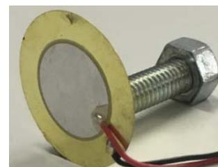
Fig. 3. Photograph of the transducer.
