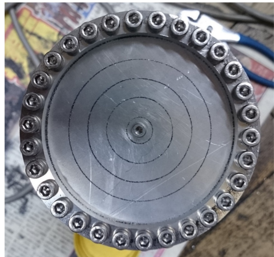
Fig. 4 Chladni figure of a vibrating plate with a rigid wall (diameter: 91mm).
