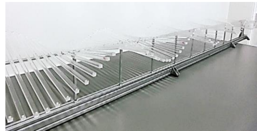
Fig. 2 View of the bare wave machine. About 100 unit cells are constructed with acrylic rods and threaded wires. A travelling wave is clearly visible.
