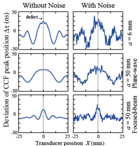
Fig. 4 Deviation of cross correlation function peak position  $\Delta\tau$  of each transmitter arrays and transmitting wave shapes.
