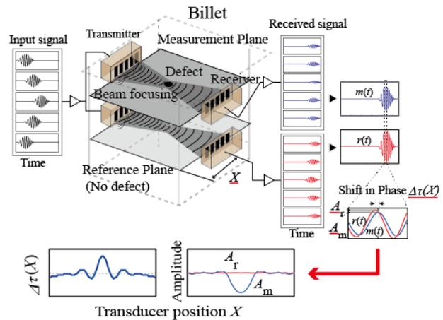
Fig. 1 Outline of defect detection inside billet by transmission method using phased array technique.
