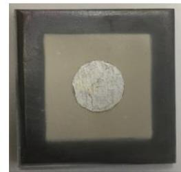
Fig.1 50μm thick BiT/TiO<sub>2</sub> film with silver top electrode on 3mm thick titanium substrate.
