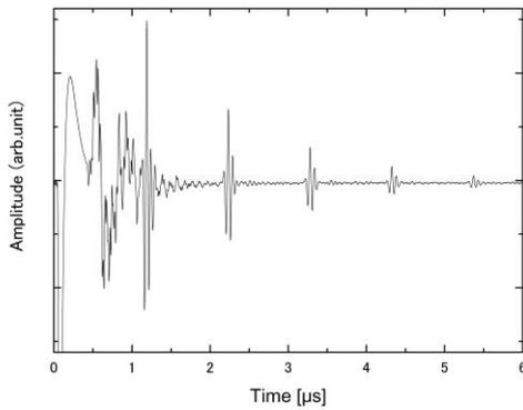
Fig.2 Ultrasonic response at 500°C in the 3<sup>rd</sup> cycle of BiT/TiO<sub>2</sub> sample fired at 400°C.
