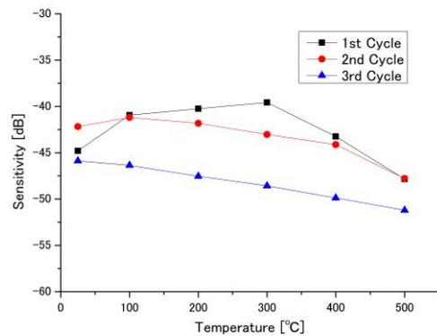
Fig.4 Sensitivity of BiT/TiO<sub>2</sub> sample at various temperatures during thermal cycle test.
