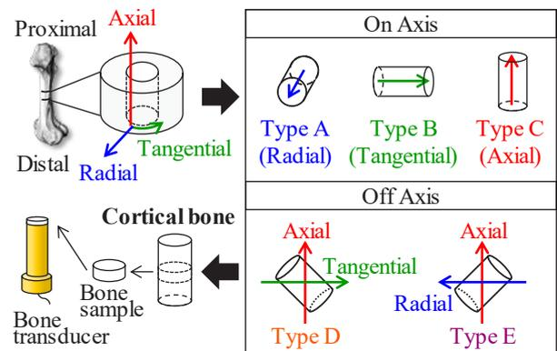
Fig. 1 Preparation of the bone transducers.
