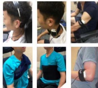
Fig. 1 Placements of the vibrator
