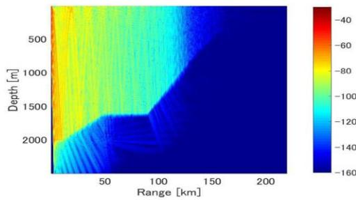
Fig. 3 Sound fields for frequency of 100 Hz SD;100 m
