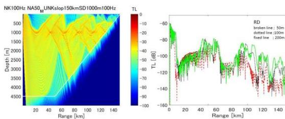
Fig. 4 Sound field and TL curve from 50 km pnt. freq; 100 Hz left) sound field right) TL curve
