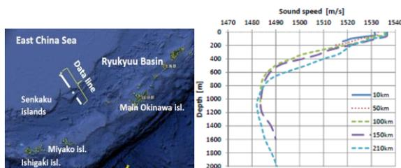
Fig. 1 Data line and Sound speed structures
