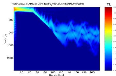
Fig. 2 Sound fields for frequency of 100 Hz
