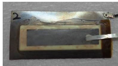
Fig. 1 Optical image of PZT/PZT piezoelectric film sensor.
