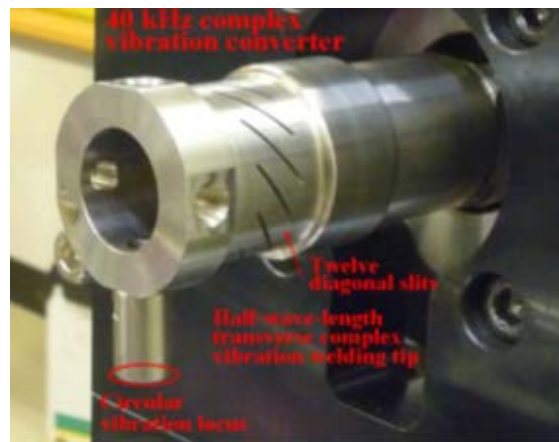
Fig. 6 40 kHz ultrasonic complex vibration welding system (SUS304) using a 30-mm-diameter, one longitudinal wave-length mode diagonal slit complex vibration converter with a half wave-length welding tip.
