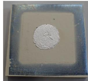
Fig. 1. Optical image of PZT/ $\text{Al}_2\text{O}_3$  sample on a 3-mm thick titanium substrate.
