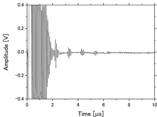
**Fig. 3.** Ultrasonic response of PZT/Al<sub>2</sub>O<sub>3</sub> sample fabricated on 3-mm-thick titanium substrate at 300°C.
