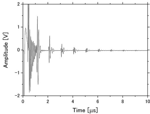
**Fig. 2.** Ultrasonic response of PZT/Al<sub>2</sub>O<sub>3</sub> sample fabricated on 3-mm-thick titanium substrate at room temperature.
