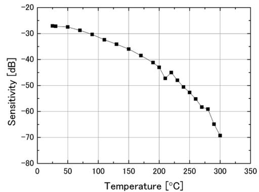
**Fig. 4.** Temperature dependence of the sensitivity of PZT/Al<sub>2</sub>O<sub>3</sub>.
