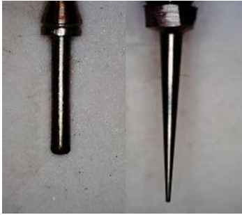
Fig. 2 The shape of poling needle, conventional needle (left) and new needle (right).
