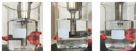
Fig. 1 The positions of the sonicator's probe used in this study.
