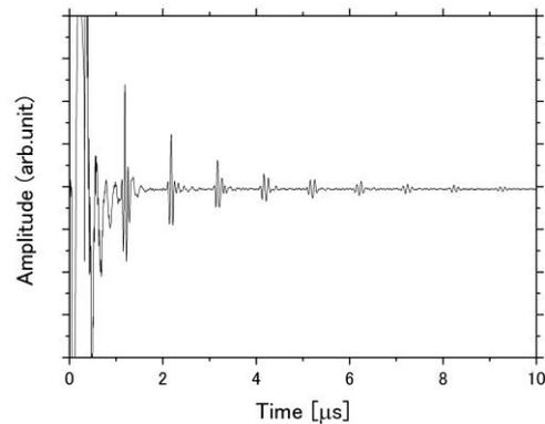
**Fig.4** Ultrasonic response of LN/BiT at RT after high temperature test.
