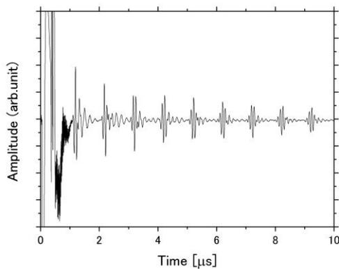
**Fig.2** Ultrasonic response of LN/BiT on 3mm thick titanium substrate at RT.
