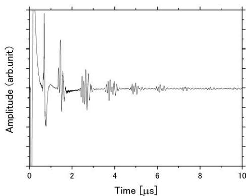
**Fig.3** Ultrasonic response of LN/BiT on 3mm thick titanium substrate at 940 °C.
