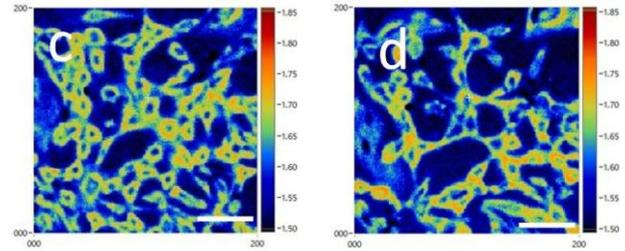
Fig. 3 Acoustic impedance image of C2C12 cells before and after HDAC inhibitor treatment. A, B: Images of 4 days after induction of differentiation before VPA treatment (A) and 5 days after induction of differentiation after VPA treatment (B) are shown. C, D: As a control, images of 4 days (C) and 5 days (D) after differentiation induction without VPA treatment are shown. Scale bars, 100  $\mu$ m.
