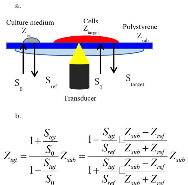
Fig. 1 Diagram of breast cancer cells observation using acoustic impedance microscope (a). Waveform parameter extraction formula (b).
