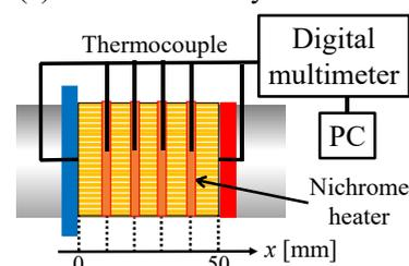
(b) Schematic of stack
