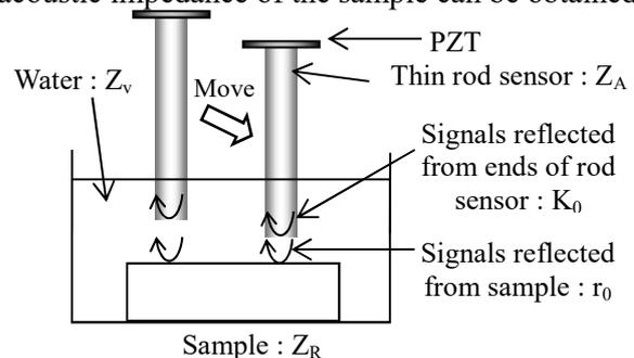
Fig. 1 Ultrasonic interference method procedure.
