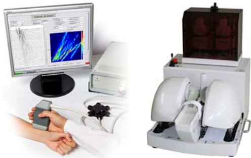
Fig. 2 The axial transmission device (left, France) and the two-wave apparatus LD-100 (right, Japan) for the radius 15, 18 .
