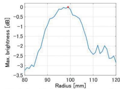
Fig. 7 Relationship between radius and maximum brightness when the target is stationary.
