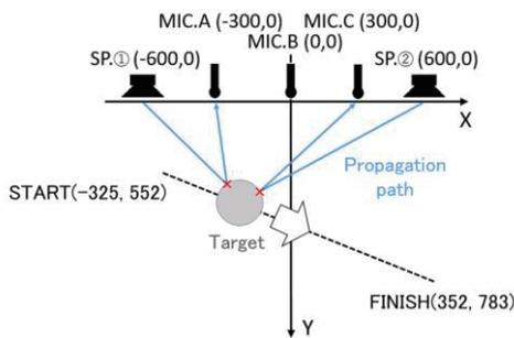
Fig. 1 Measurement configuration.
