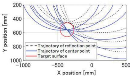
Fig. 3 Estimation of center position.
