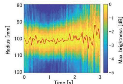
Fig. 8 Relationship between radius and maximum brightness when the target is moving.
