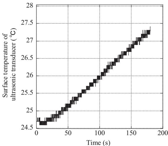
Fig. 3 PZT surface temperature of ultrasonic transducer measured by thermocouple.
