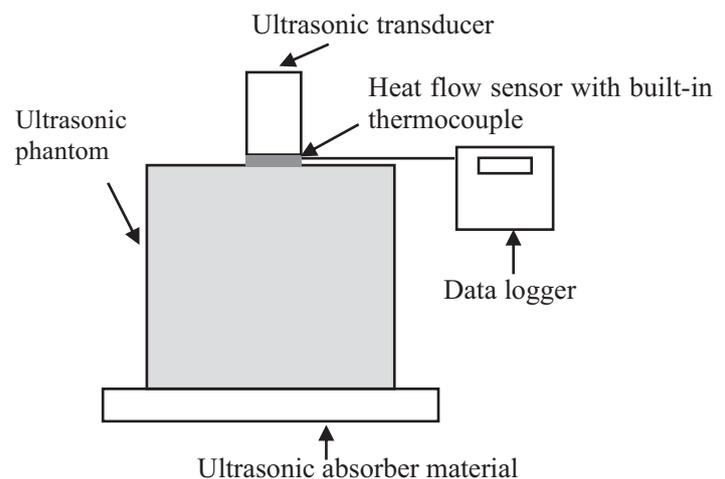
Fig. 1 Experimental system for measuring heat flow and temperature.
