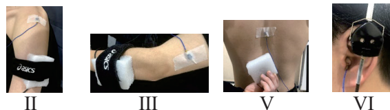
Fig. 3 Locations of the BCU stimuli and the accelerometer: II. Pinna, III. Cartilago thyroidea, V. Thoracic vertebrae, VI. Cartilago costalis. In each location, the accelerometer was placed so that the distance between the vibrator and the accelerometer was 13 cm.
