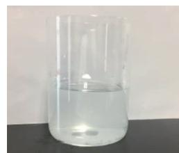
Fig. 2 Appearance of the solution treated by ultrasound for 30 min in the presence of a lead electrode.
