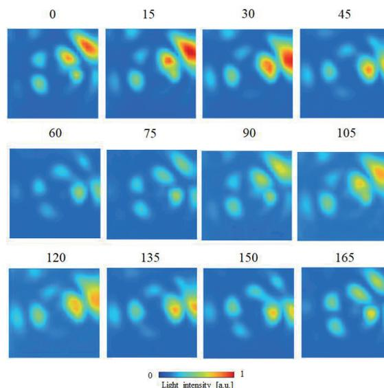
**Fig. 3** Distributions of the transmitted light intensity with ultrasound excitation at each polarization directions ( $\theta = 0^\circ$  to  $165^\circ$ ).
