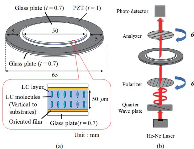
Fig. 1 An ultrasound large-aperture liquid crystal lens. (a) Configuration and (b) experimental setup.
