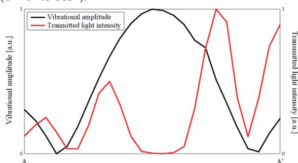
**Fig. 4** Distributions of the transmitted light intensity (red) and vibrational amplitude of the glass substrate (black) at 35 kHz along line A–A' in **Fig. 2**.
