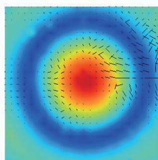
**Fig. 5** Distribution of the liquid crystal molecular orientation and the vibrational distribution.
