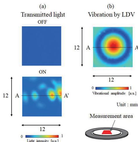
Fig. 2 (a) Distributions of the transmitted light intensity without and with ultrasound excitation at the polarization directions  $\theta$  of  $45^\circ$  and (b) the distribution of the vibrational amplitude of the glass substrate at 35 kHz.
