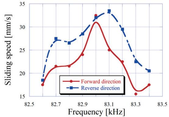
Fig. 5 Sliding speed as a function of driving frequency (driving voltage  $V_{L1}$ : 200 V<sub>pp</sub>,  $V_{B1-2}$ : 200 V<sub>pp</sub>, phase difference  $\phi$ :  $\pm 90$  deg., preload: 0.16 N)
