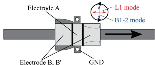
Fig. 2 Driving principle of the proposed USLM
