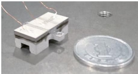
Fig. 3 Prototype of the stator transducer
