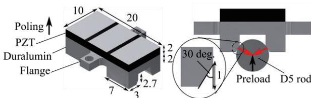
Fig. 1 Schematic diagram of the proposed USLM stator transducer
