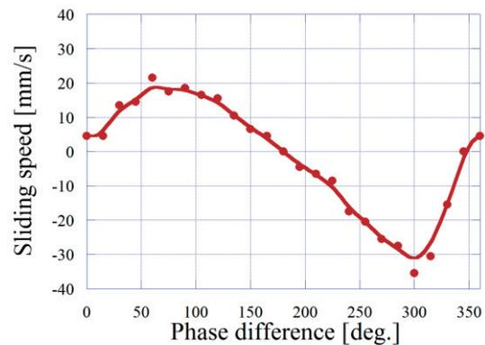
Fig. 6 Sliding speed as a function of phase difference  $\phi$  (drive frequency: 83.0 kHz, driving voltage  $V_{L1}$ : 200 V<sub>pp</sub>,  $V_{B1-2}$ : 200 V<sub>pp</sub>, preload: 0.16 N)
