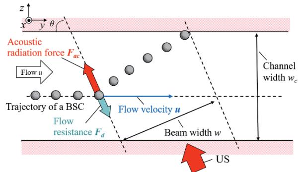
Fig.1 Trajectory of a BSC in flow under ultrasound exposure.
