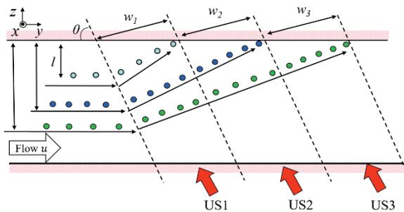
Fig.3 The model of the retention of the acoustic field with multiple focal points.
