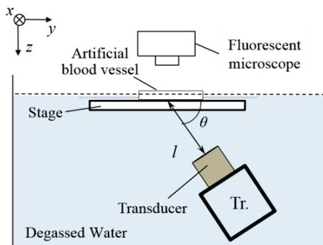
Fig.2 Experimental setup to expose ultrasound to suspension of BSCs in an artificial blood vessel.
