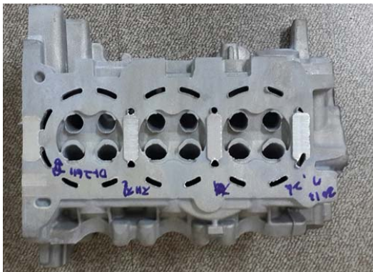
Fig.2 Sand cast cylinder head of AZ-type Eco-Mg by using general sand mold
