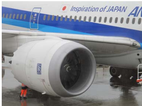
Fig.3 First application of NIMS advanced SC superalloy was made in Rolls-Royce Trent1000 engine powering Boeing 787.
