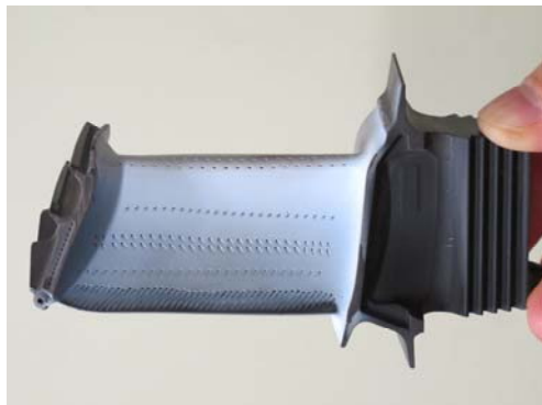
Fig.4 An example of Rolls-Royce hollow turbine blade with thermal barrier coating and holes for film cooling.
