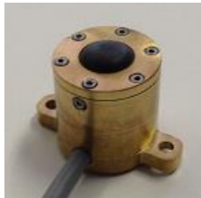
Fig 3: sensor for in-situ measurement of mold
