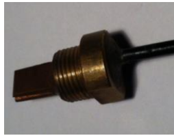
Fig 2: sensor for sand detection
