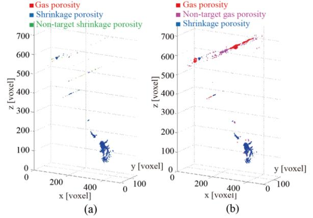
Fig. 2 Results of the porosity discrimination. (a) Before the blister test. (b) After the blister test.
