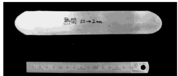
Fig.4 Appearance of Al-2%Li-2%Cu-1.5%Mg-0.10%Zr alloy plate hot rolled in 90%.
