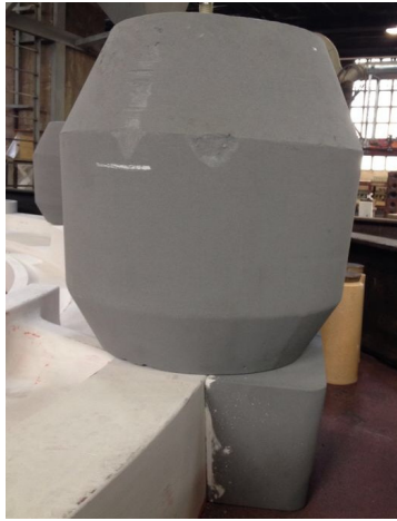
Fig. 3. Mini-riser with an 34.500cc exothermic padding.
