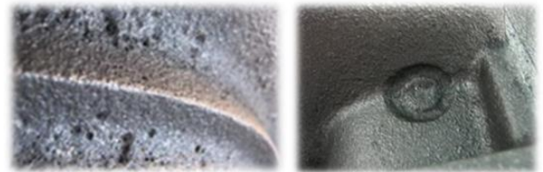
Fig.4 Fluorine-induced surface defects
