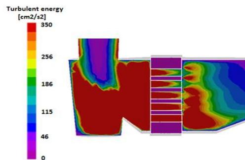
Fig. 2 Turbulence intensity – Variant A, time 0.6 sec.
