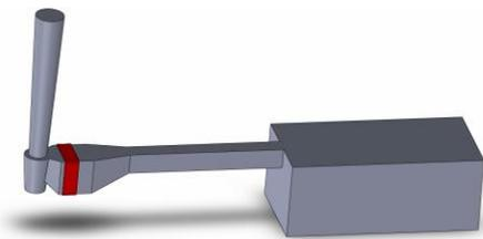
Fig. 1 Gating system with the filter location
