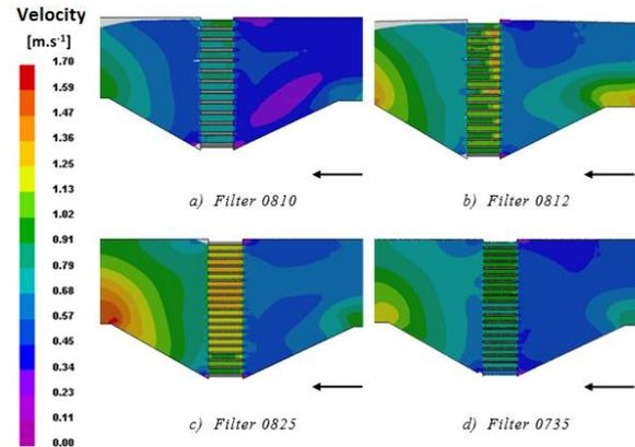
Fig. 5 Melt velocity – time 0.65 sec.
