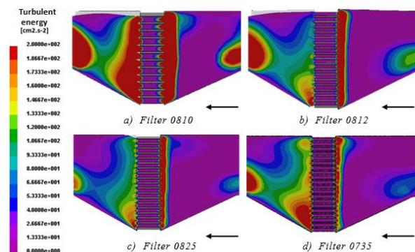
Fig. 6 Melt turbulence – time 0.65 sec.
