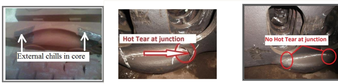
Fig4 External chills to arrest hot tears Fig 5 Hot tear before and after in real casting
