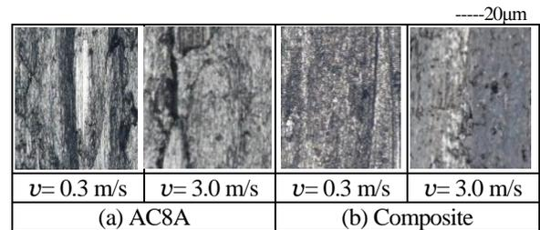
Fig. 4 Worn surfaces of the disk specimens after wear test.
