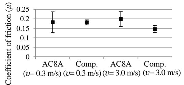
Fig. 3 Coefficient of friction of AC8A alloy and composite under wear test.
