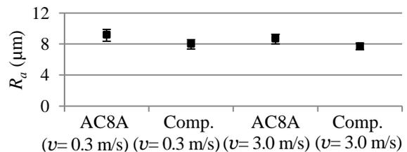
Fig. 5 Surface roughness of disk specimens after wear test.
