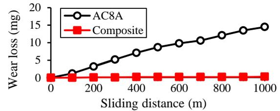
Fig. 2 Relationship between sliding distance and wear loss of AC8A alloy and composite.
