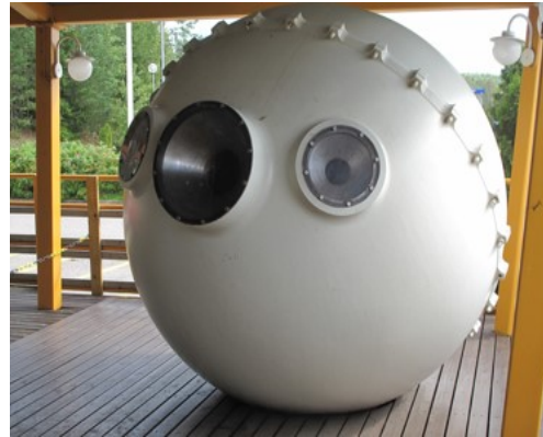
Figure 2: The sphere's halves joined together with bolt joints. The remaining hemisphere is exhibited at the Lokomo steel foundry which is nowadays called TEVO Lokomo Ltd. [7]
