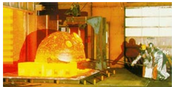
Figure 1: The heat treatment of the sphere halve at the Lokomo steel foundry. [3]
