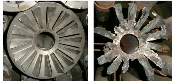
Fig. 1 Diffuser before and after failure.
