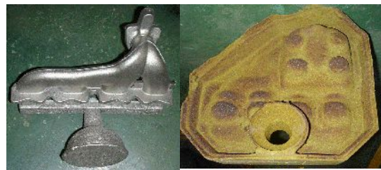
Fig.3 Steel castings (left) produced using the lightweight shell mold (right)
