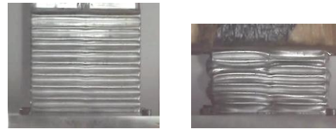
Fig. 6 Photos of the crash absorption component with the wavy design before and after the drop-weight test.
