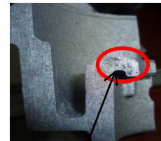
Fig.11 Micro Shrinkage on Valve seat
