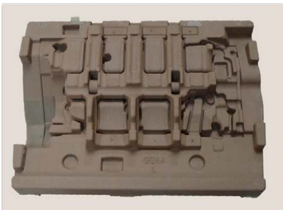
Figure 3: Coating Application core package process Eisenwerk Brühl Germany
