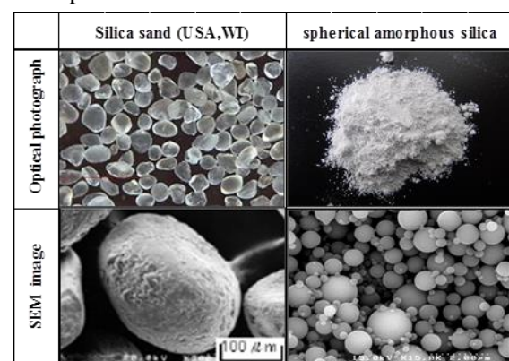
Fig. 1 Optical and electron photomicrographs of natural silica sands and acid spherical amorphous silica fillers.
