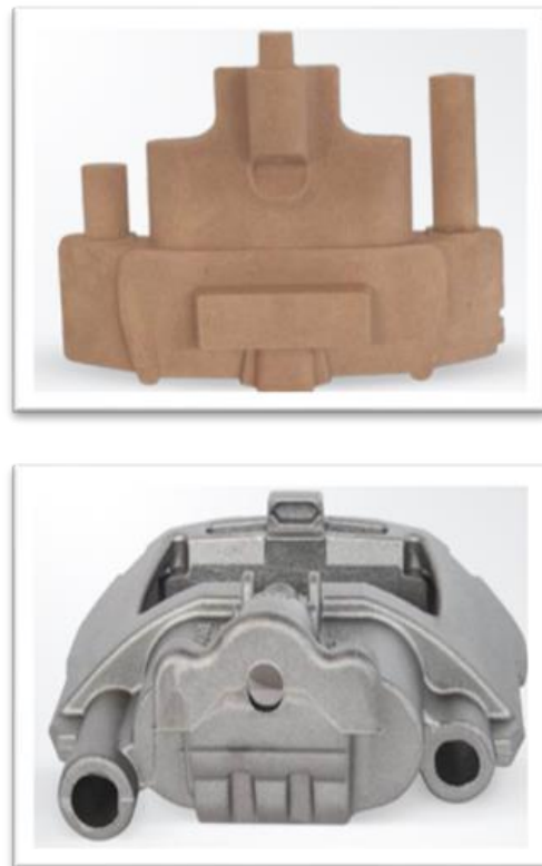
Fig. 1 Uncoated core and casting poured with uncoated core
