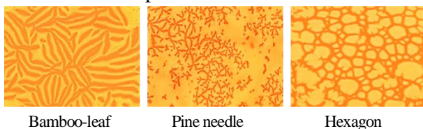
Fig. 1 Molten cast iron surface pattern in gray iron.
