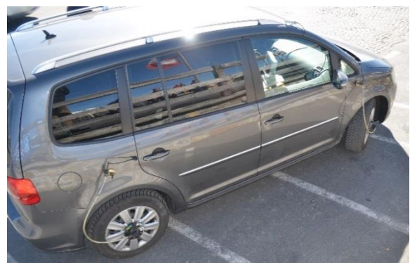
Figure 1. VW Touran wheels instrumented for road testing.
