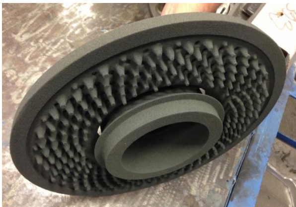
Figure 3. Photograph of 3D printed core with as-cast holes in brake faces.
