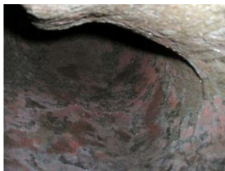
Fig.4 Appearance of the applicable part after Sand Cleaning (After the shot-blast)
