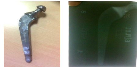
Fig.6 Actual femur implant casting along with radiograph
