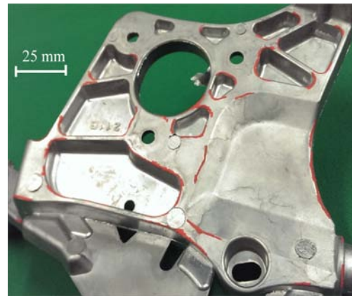
Fig. 4 Transcribed heat-checking observed in the part on the movable-die side after 120,000 shots. Enlarged view of the square area enclosed by the dotted line in Fig.3 (a).
