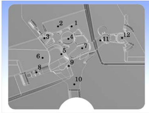
Fig. 2 Points 1 through 12 used in stress calculation for the movable-die surface.
