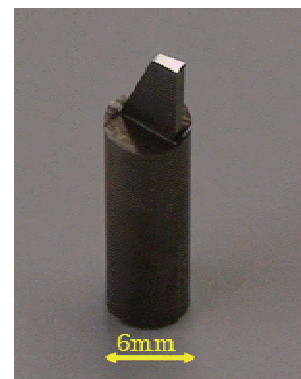
Fig.1 Used tool with low bending rigid
